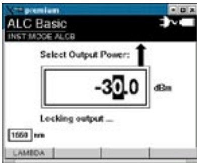
1. ALC Basic Mode: This easy-to-use automatic level control mode needs only the output power, that's it
