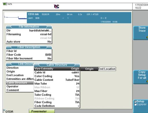
Figure 3: Documentation using the MTS/T-BERD Platforms
